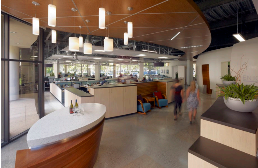
The natural ventilation continues through the open workspaces, where there are overhead HVLS fans and desks with intentional low cubicle walls. The passive airflow “breathes” through the building when windows and doors open on opposite sides of the office.
